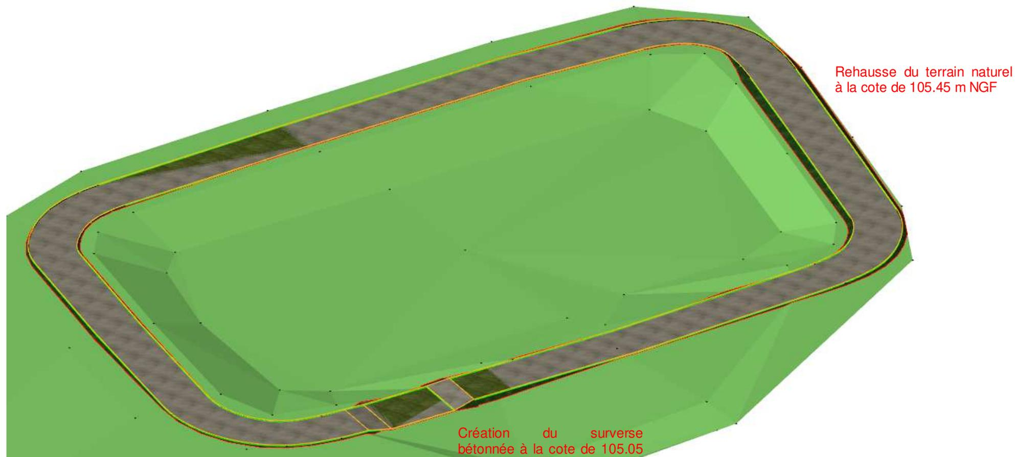
**Fig. 11. MODIFICATION A APPORTER AU BASSIN DE RETENTION DU PARC DE LA NAUZETTE**
